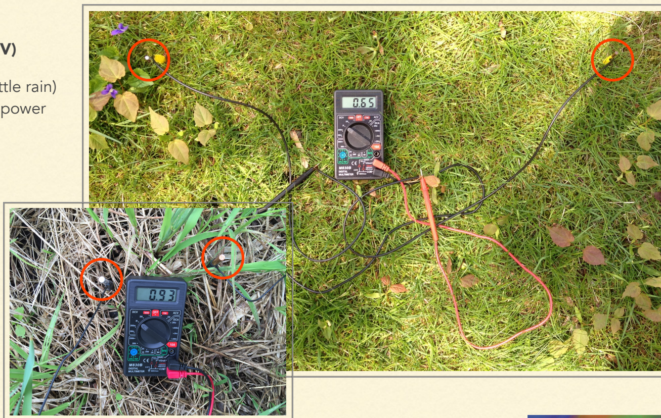
Lawn battery (summer). INSET: Marsh mud battery. (Circles show position of electrodes.)
